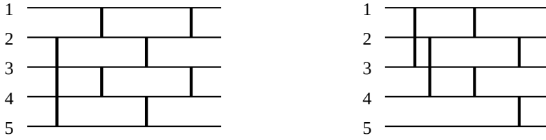
Fig. 2. The network F_5 has depth 4 and the optimal simple correction network for N = 5 has depth 3.
